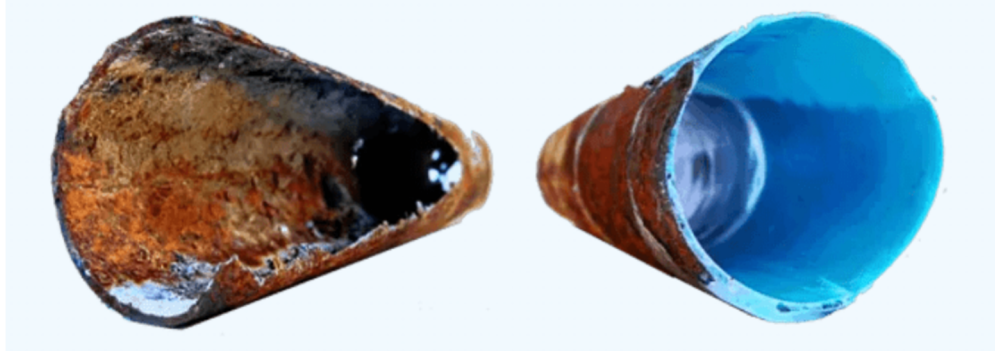
Figure 1: Before and After Pictures of Pipe Rehabilitated with CIPP Lining System (image taken from piperestorationsolutions.com)
